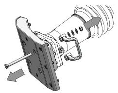
▶ Remove the tamping foot, the fasteners and the handle.
