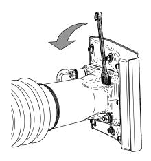
▶ Loosen the four nuts of the tamping foot.
