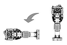
▶ Lay the tamper down on its side.
