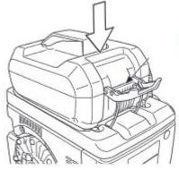
▶ Push the battery pack down and hook in the battery fastener.
