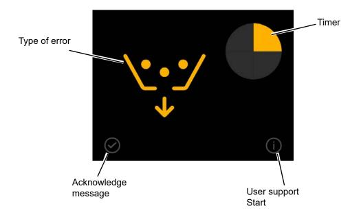
The user assistant provides an intuitive interface that guides the user through the work steps necessary to eliminate a fault. "Info" displays a QR code. The user can scan this code to access the spare parts list and the operating instructions of the machine.
