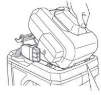
▶ Tip the battery back and insert the claw into the battery hook.
