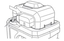
▶ Remove the protective cap from the battery connector and insert the power cable.
